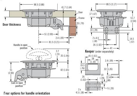
Install keeper using 2 x M4 (No. 8) screws (not supplied)
